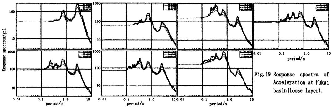
Fig.19 Response spectra of Acceleration at Fukui basin(loose layer).
