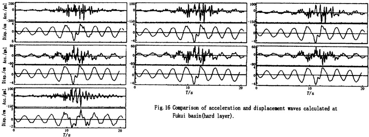
Fig.16 Comparison of acceleration and displacement waves calculated at Fukui basin(hard layer).
