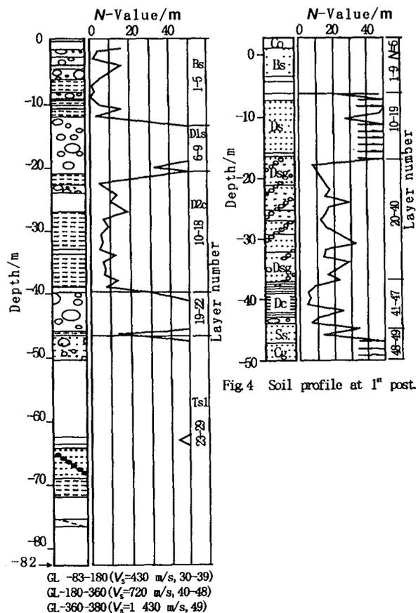
Fig. 3 Soil profile at 2<sup>nd</sup> post.
