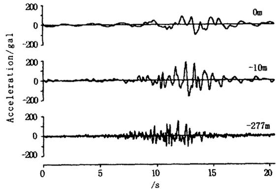
Fig. 12 Calculated waves by SHAKE.
