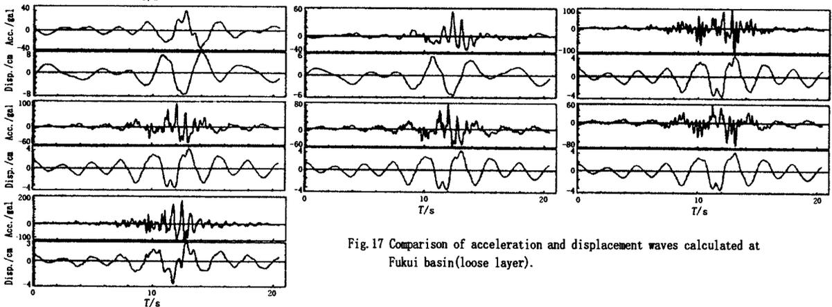
Fig.17 Comparison of acceleration and displacement waves calculated at Fukui basin(loose layer).
